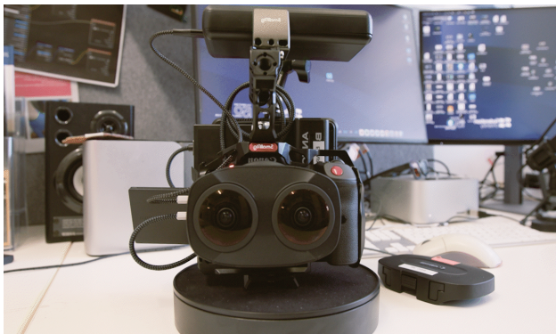
VR180 production rig: Canon R5C with stereo dual fisheye lens
